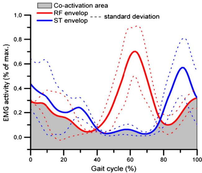
Fig. 1. Illustration of the co-activation index computation (co-activation area) for a typically developing child limb in the rectus femoris (rf)/semitendinosus (ST) muscle couple.
